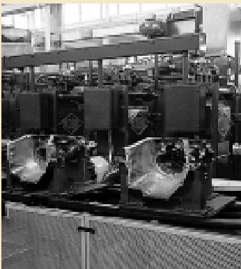
5,000 psi design pumping water and soluble oil for deburring machined metal parts.
