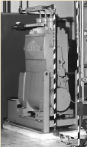
30,000 psi design pumping straight water @ 13,000 psi for high pressure jet cutting.
