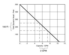
The curve above shows that with a 100 foot change in head, the capacity varies only 2 gallons per minute. You get a virtually constant flow over wide pressure variations to ensure reliable system operation.
