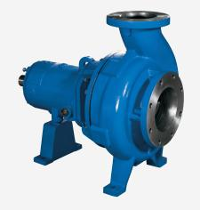
Pentair's ANSI B73.1 standard dimensional process pump is a versatile workhorse. This pump comes in a variety of materials of construction from 316 SST to titanium. Capacities to 5,600 gpm with heads to 550 feet, this pump is also ideal for many chemical and transfer fluid applications.
