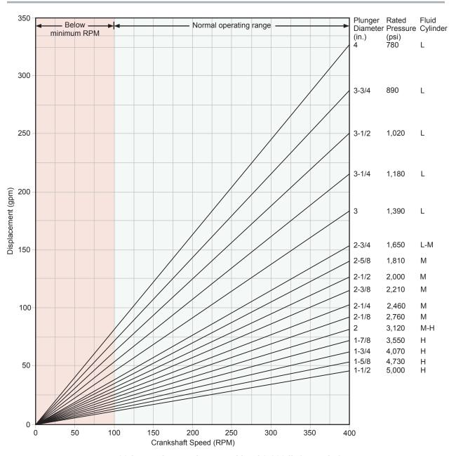
5.00-in. stroke, maximum rod load 9,800 lb (4,445 kg)
