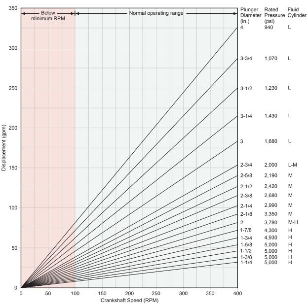
5.00-in. stroke, maximum rod load 11,870 lb (5,384 kg)
